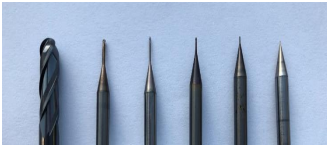
Figure 1 \varnothing 6 tool used in micro-machining and \varnothing 1 , \varnothing 0.6 , \varnothing 0.5 , \varnothing 0.3 and \varnothing 0.15 micro-tools used in micro-machining seen respectively in the picture.
